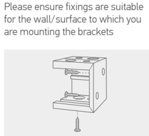
Open the gate of the box brackets and slide the headrail into position then snap the brackets closed.
